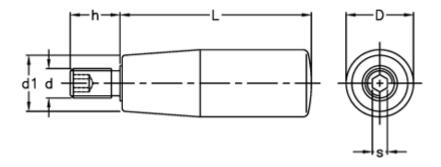
$$\begin{array}{ll} D & = 14 \\ d1 & = 11 \\ d \ 6g = M6 \\ h & = 10 \\ L & = 28 \\ s & = 3 \end{array}$$
